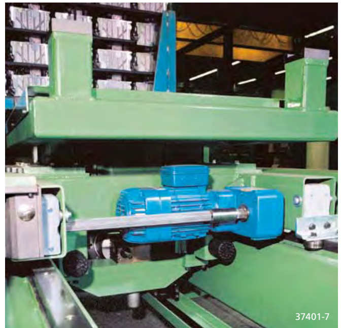
Line-fed KBF motor used as a shuttle drive for smoothly transporting goods in a storage system
