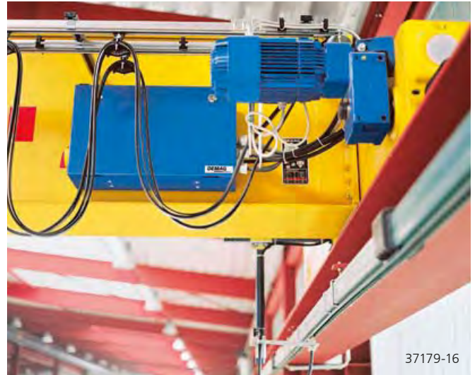
A crane end carriage driven by an offset geared motor
