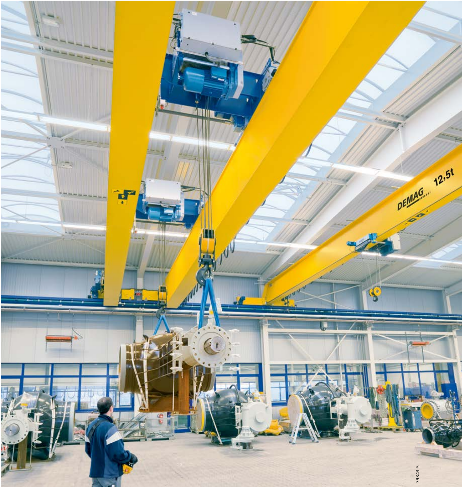
The double-girder design provides for particularly high load capacities and sensitive load handling thanks to infinitely variable speed control in three axes, including tandem operation
