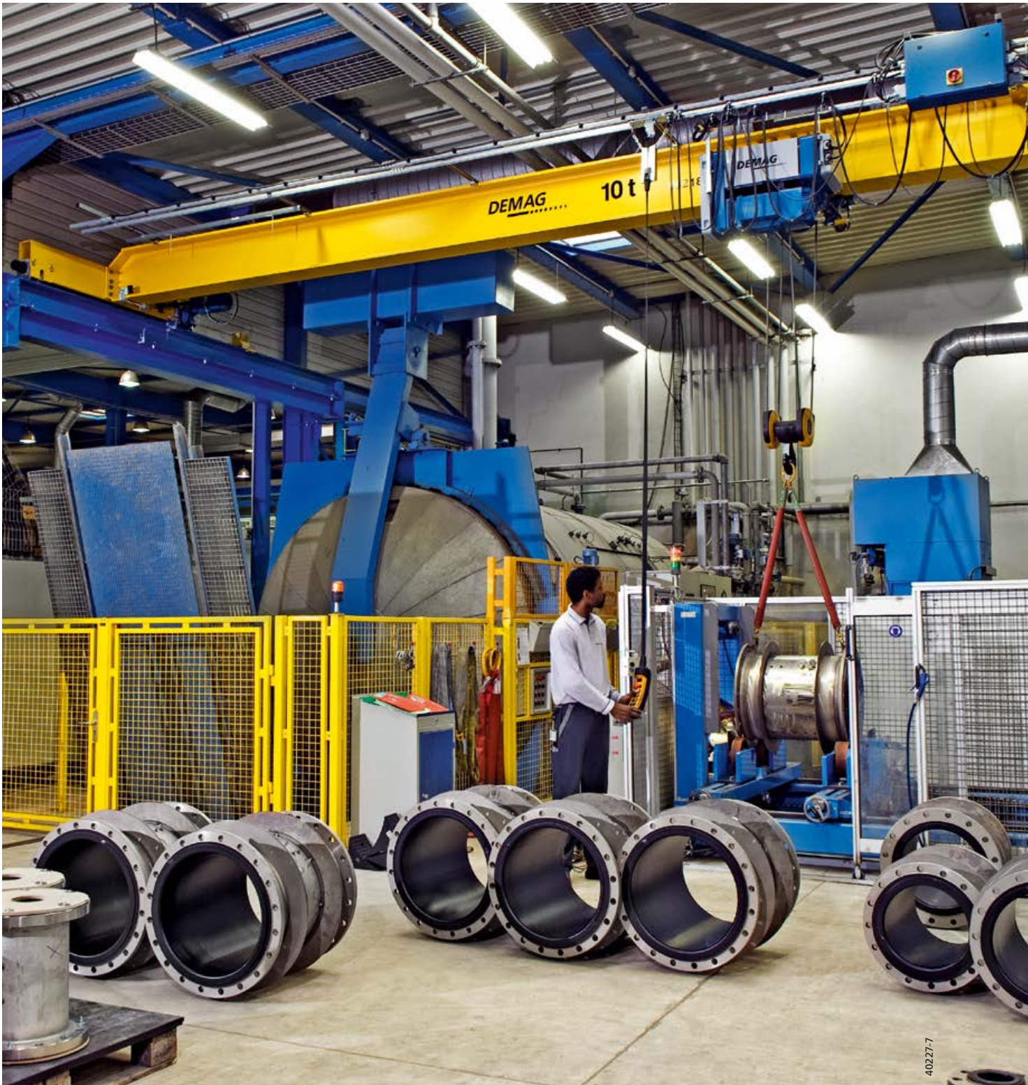
Single-girder EPKE overhead travelling cranes can be fitted to order with either DR rope hoists or DC chain hoists
