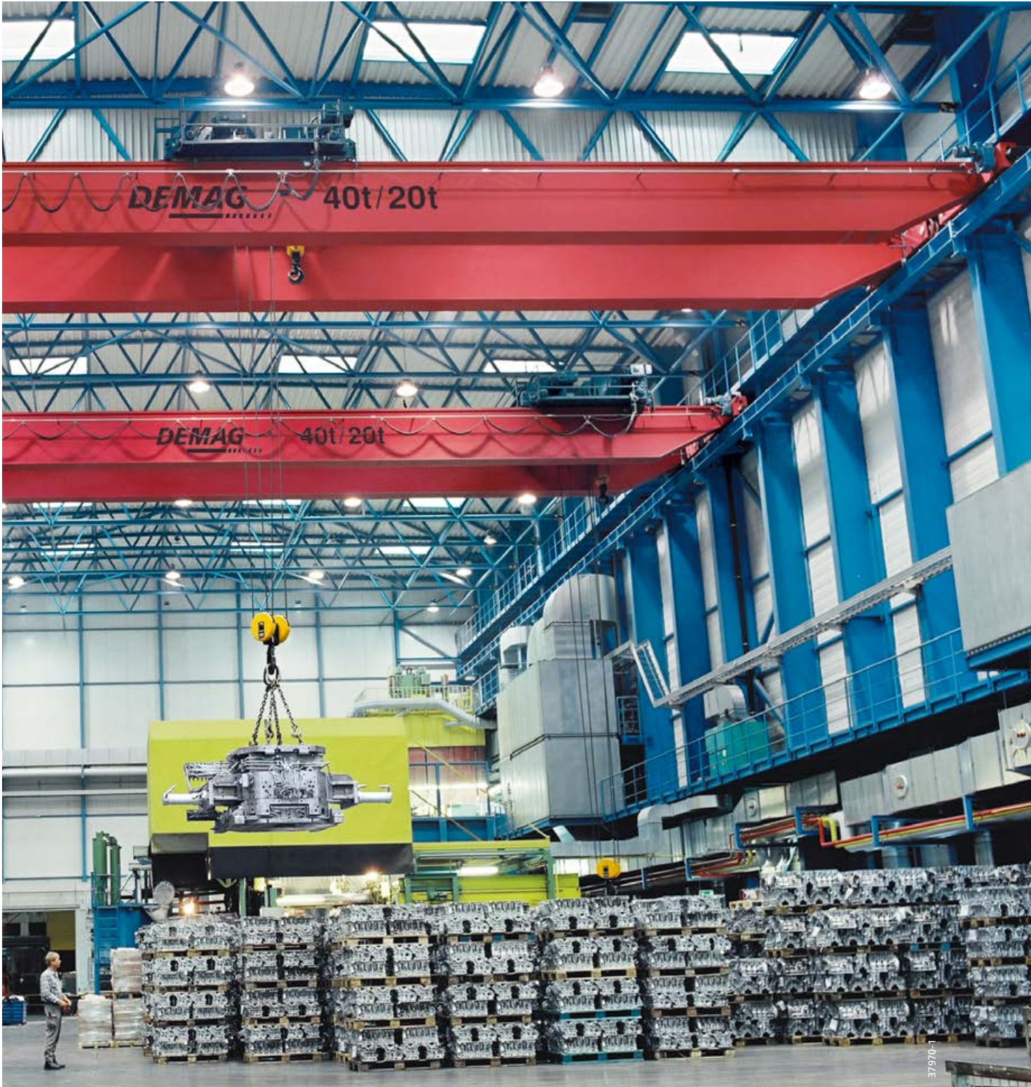
Double-girder overhead travelling crane with tandem end carriages for transporting and turning engine blocks
