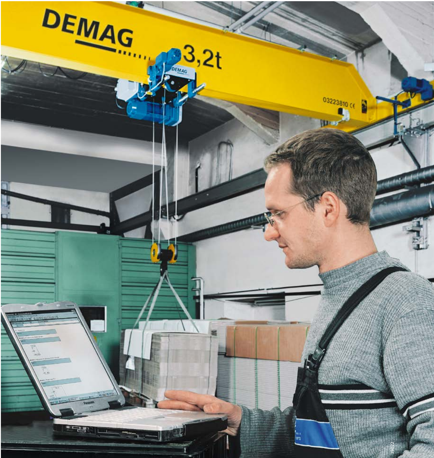
Crane system data can be read out to facilitate scheduled maintenance and service
