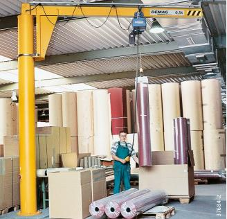
This slewing crane is the universal solution for a load range up to 5,000 kg. The low-headroom jib provides for particularly long hook paths for an unlimited slewing range. The jib can also be powered by an optional electric slewing drive for ease of operation.
