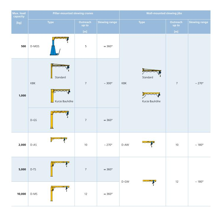
The crane types shown on the following pages are designed for indoor operation as standard. Designs
