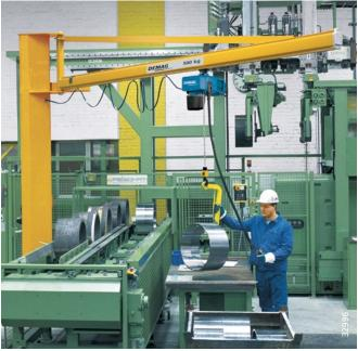
KBK slewing jibs feature high load capacities and outreach in relation to their deadweight. The low weight enables the jib to be moved easily and the use of KBK hollow section rail as the crane girder provides for very low travel forces.
