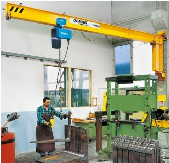
With its low-headroom jib and high load capacity, the D-GW wall-mounted slewing jib is suitable for a wide variety of applications. The crane is designed for use with Demag chain hoists or Demag rope hoists.
