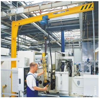
The light-weight design and low-headroom jib make this pillar-mounted slewing jib crane suitable for universal applications in a load range up to 2,000 kg.
