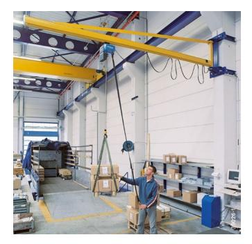
Wall-mounted slewing jibs do not take up any floor space. They are mounted on load-bearing concrete walls, pillars, or existing machinery and installations. They are particularly easy to install, since the bracket is supplied ready to be fitted as a unit, which eliminates any complicated alignment work. KBK wall-mounted slewing jibs are suitable for a load range up to 1,000 kg.
